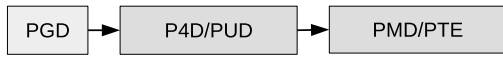
(b) If most entries are for 4 KiB pages, then density is best pushed closer to the PTE, and so the PGD is left sparse.
