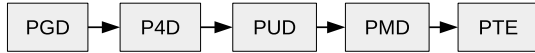
(a) Five-level page tables introduce a new layer, P4D, to increase virtual-address size from 48 to 57 bits.
