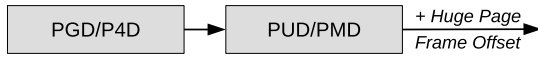
(c) If most PMD entries down a path are to huge pages, then all levels can be made dense even with an odd number of layers.
