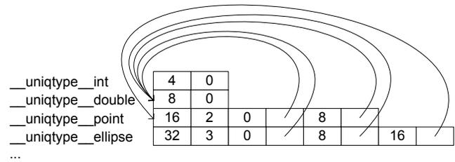
**Figure 7.** Our `uniqtype` representation (slightly simplified) of the ellipse and types it uses: pointer arcs represent containment, and the fields preceding pointers are the offsets of the contained subobject; other variants (not shown) encode arrays, functions, pointers, etc.
