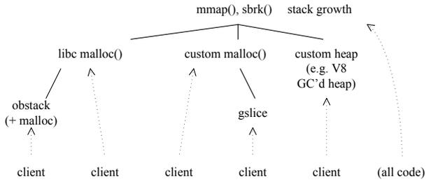
**Figure 4.** Allocator tree in a large C/C++/JavaScript program
