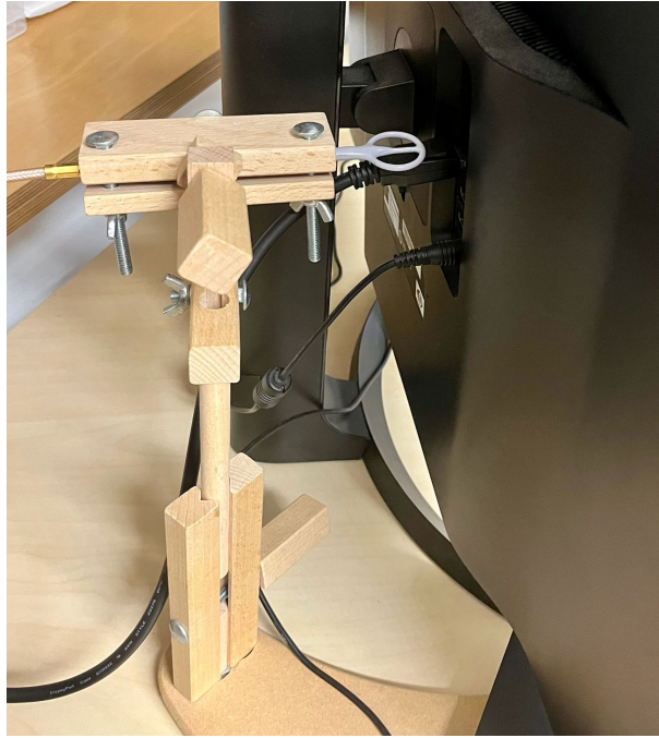
Figure 5.1: Near-field H-probe held near the DisplayPort cable connector
