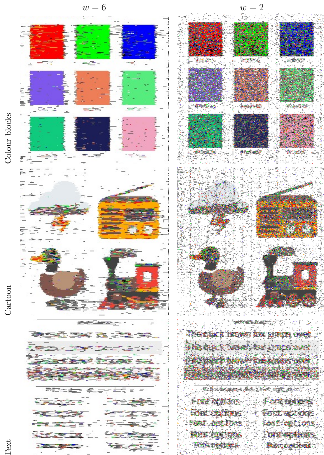
Figure 4.11: Effect of the window size w on windowed incoherent-averaging decode quality, at a fixed frame count, for three content types.
