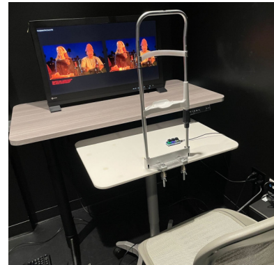
Fig. 12. Physical hardware setup for the XR-DAVID data collection. Participants used a chinrest to fix their distance from the display at 0.73 m (two display heights) and used a 3-key keyboard to record their choices.
