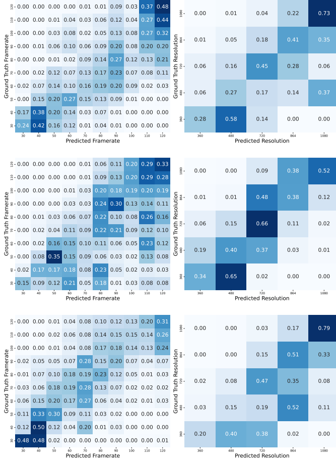
Fig. 7. Confusion matrices for frame rate and resolution prediction, showcasing our 3-fold cross-validation. These results correspond to the best-performing model configuration ("Full model" in Table 1). Each row is normalized by the total number of samples per class.
