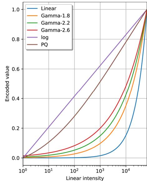
FIG. 7: TFs used in our experiments to map linear color values to the encoded values, suitable for CV methods.
