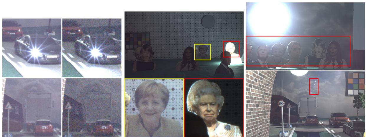
(a) Patches of the **night** illumination (right column) captured with exposure time  $t = 1/150$  secs and gain  $g = 16$ , compared to **uniform** illumination (left column).
