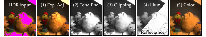
Fig. 3. Generic tone mapping operator. Here, we show the operations applied to the HDR “Toys” image in our generic tone mapper. Note that HDR content cannot be accurately shown here, so we visualize out-of-gamut pixels in the input HDR image in magenta.
