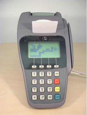
Figure 8: Modified Chip and PIN terminal, playing Tetris
