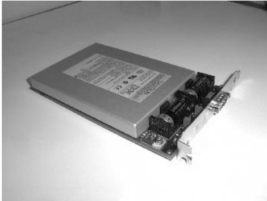
Fig. 1. – the IBM 4758 cryptoprocessor (courtesy of Steve Weingart)
