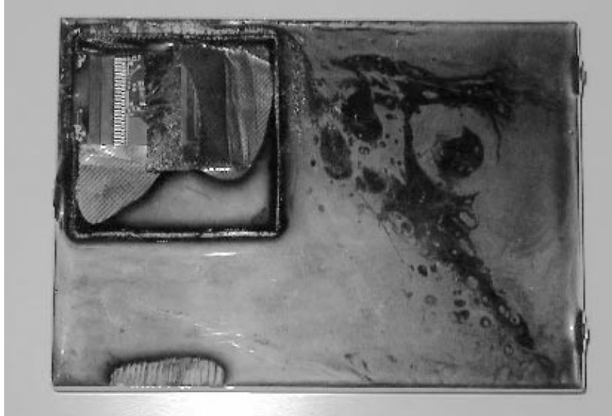
Fig. 2. – the 4758 partially opened – showing (from top left downwards) the circuitry, aluminium electromagnetic shielding, tamper sensing mesh and potting material (courtesy of Frank Stajano)
