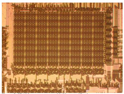
Figure 5. SRAM memory array with 80x magnification
