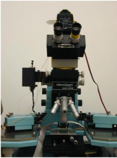
Figure 6. Wentworth Labs MP-901 manual prober with Vivitar 550FD photoflash lamp mounted on top
