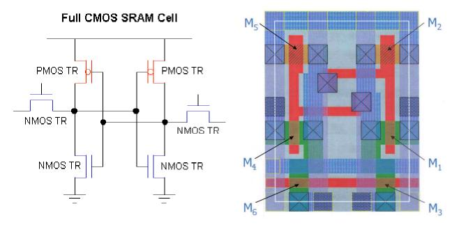
Figure 1. Structure of six-transistor SRAM cell
