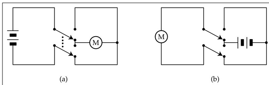
**Figure 25.3:** Hazard elimination in motor reversing circuit
