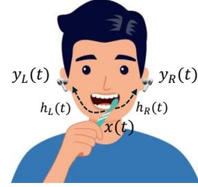
**Figure 6: The signal propagation model of SmarTeeth. The in-ear microphones can capture binaural toothbrushing sounds in two ear canals.**
