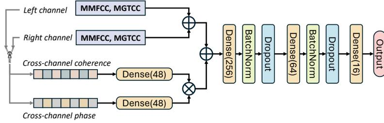
Figure 10: The deep learning model structure of SmarTeeth.
