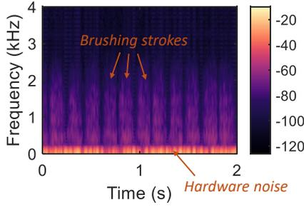
**Figure 5: The spectrogram of in-ear toothbrushing sounds. Most sounds are distributed below 2.5 kHz, and the hardware noise is below 100 Hz.**
