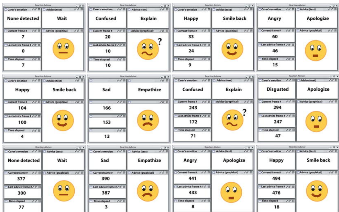
Fig. 7 A sequence of screenshots from the reaction advisor. Each screen communicates to the user the current frame number, the last time a suggestion was made and the time elapsed since then, the current inference and a recommended action to take (both textual and graphical)
