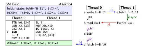
intervention (DDI), an optimisation allowing cache lines to be migrated directly from one thread's (data) cache to another. The line could be migrated from Thread 0 to Thread 1, then pushed past Thread 1's Point of Unification, making it visible to Thread 1's instruction memory without ever making it visible to Thread 0's own instruction memory. The lack of coherence between instruction and data caches would make this observable, even in multi-copy atomic machines.
