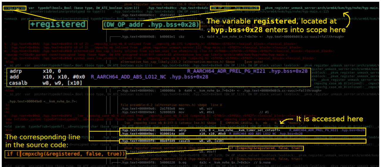
Figure C.1: Fragment of the evaluated debug information from pKVM, displayed using HTML. The code fragment is accessing a static variable registered , located in the .bss section. The output displays the program instructions (white), interleaved with parts of the debugging information. The descriptions of variables when they enter the scope are green, the corresponding lines in the source code are orange, relocations are purple.
