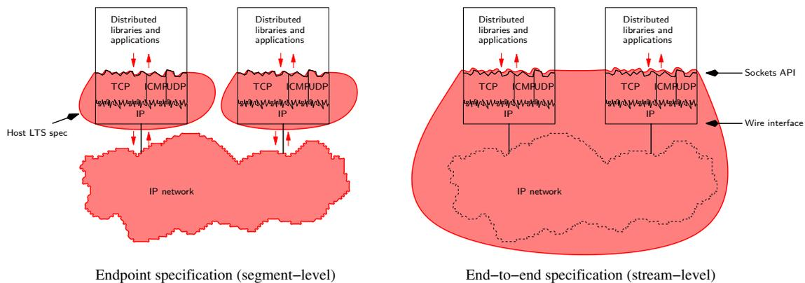
3. One could give an endpoint specification for the network interface only, as shown on the left below. This would aim to capture the wire protocol in a pure form, defining what the legal sequences of message input and outputs are for a single host.
