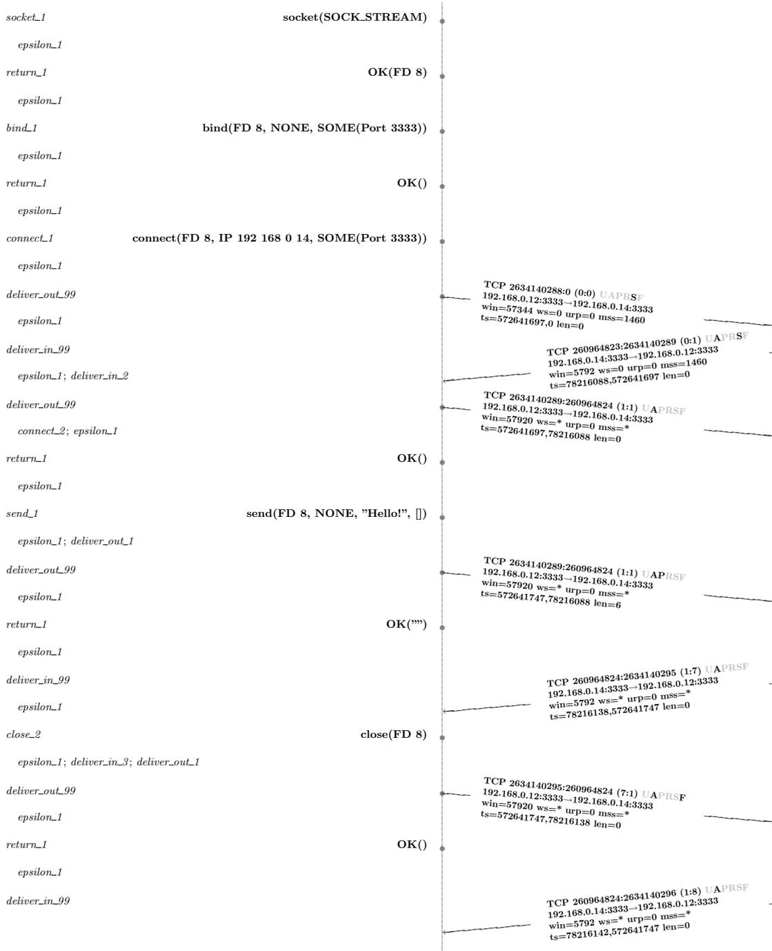
Figure 7: Sample checked TCP trace, with rule firings – connect() end
