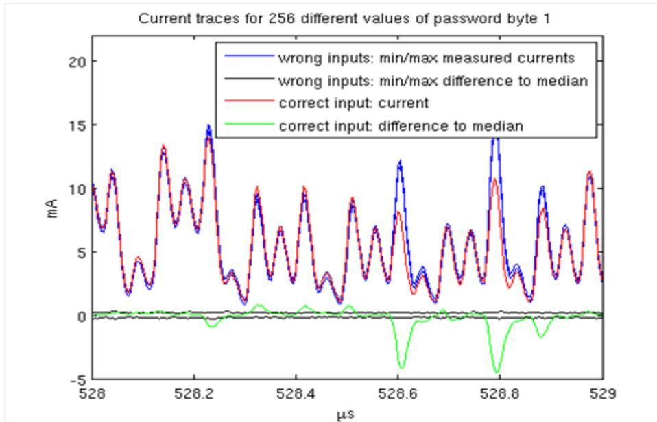
Fig. 4. SPA attack on the MC68HC908AZ60A microcontroller: plotting the intensity for all 256 possible values of a password-byte it is possible to determine the out-lier which corresponds to the correct byte; figure from [3]
