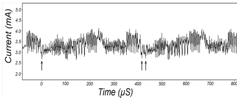
Fig. 3. Simple Power Analysis on DES encryption: the arrows mark the moments when registers C and D are rotated; figure from [4]
