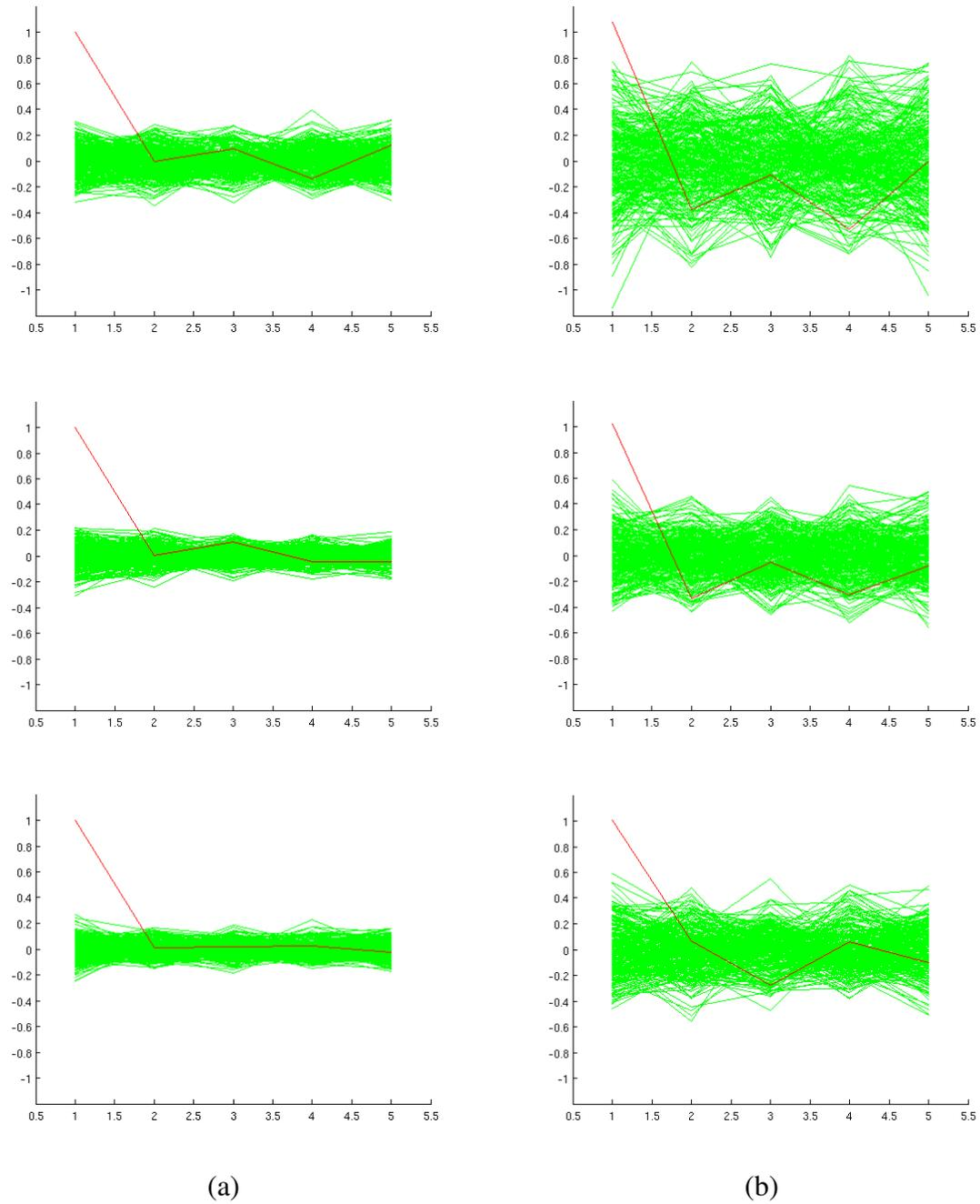
Fig. 10. Results of CPA (a) and DPA (b), for  $m=100$  (top),  $m=1000$  (middle) and  $m=10000$  (bottom). The X-axis represents the 5 iterations of each encryption operation in our algorithm; the Y-axis represents the amplitude of the correlation for CPA and the amplitude of the differential trace for DPA
