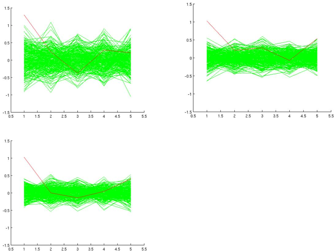
Fig. 8. Results of our DPA attack for different values of  $m$ ; on the X-axis we represent the 5 iterations of an encryption operation; the Y-axis represents the amplitude of the differential trace
