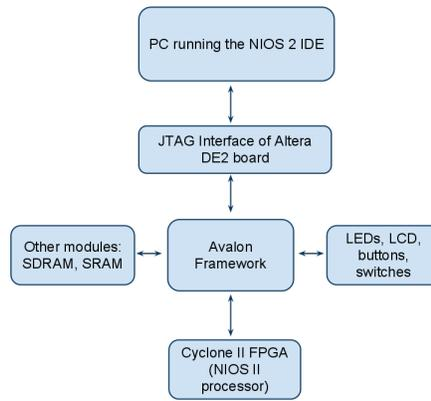
Fig. 1. Diagram of data flow using the Avalon framework on the Altera DE2 board
