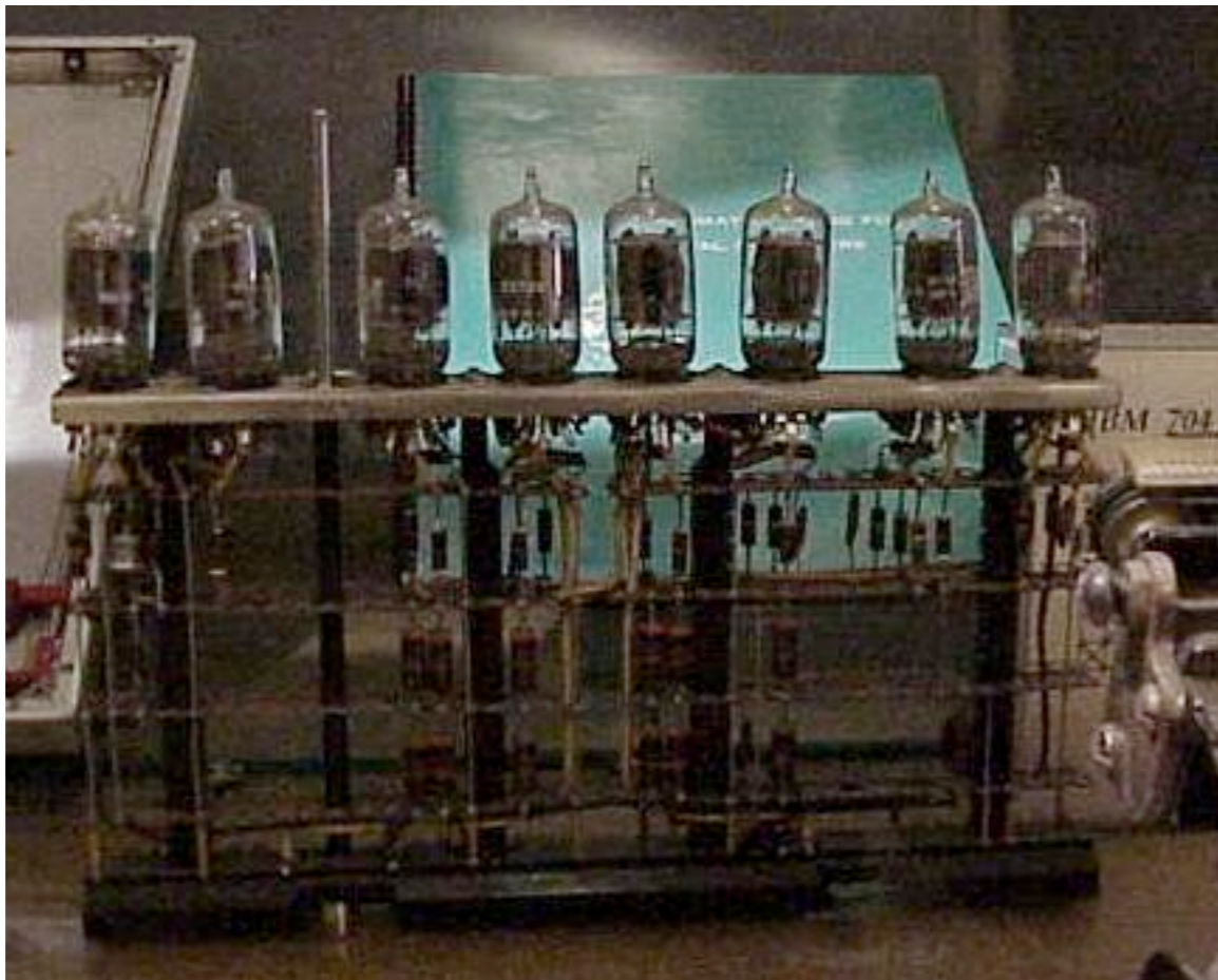
One of about 4000 Logic Modules for an IBM 704 Computer (1954). [photo: http://infolab.stanford.edu/ ]
