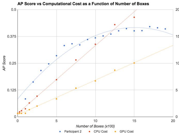
Figure 4. Demonstrates the tradeoff between AP score and computational cost for the entire pipeline (objectness and classification).
