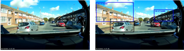
Figure 3. An example of a difficult image and its corresponding annotation. It is not clear where one row of houses ends or another begins. Also, while there are clearly three visible cars in the image, what about the other ones that are almost completely obscured and the ones that are very small. Finally, there is a church at the end of the street that, again, is mostly obscured.
