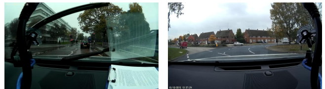
Figure 2. Two sample images from our dataset, demonstrating its particular difficulties. These images show the distortion and glare caused by the windshield, the effects of weather, and that many of the objects to be detected are extremely small.
