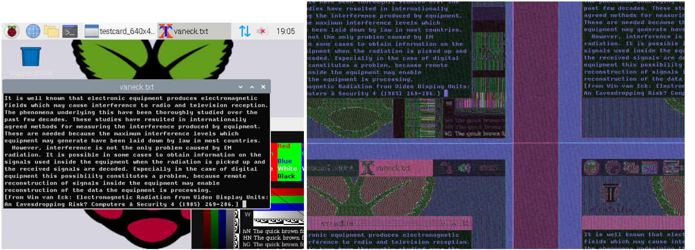
Fig. 1. Displayed 640 \times 480 @ 60 Hz test image (left), and eavesdropped 800 \times 525 -pixel frame a[n] (right), recorded at f_c = 350 MHz, after resampling, frequency alignment, periodic averaging of N = 30 frames, and HSV demodulation, but prior to frame alignment.
