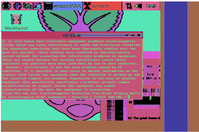
Fig. 5. The result of cycle detection. Note how the words “vaneck.txt” and “Wastebasket” become readable, which in Fig. 4 remained unrecognizable within the surrounding TMDS-balancing cycles.
