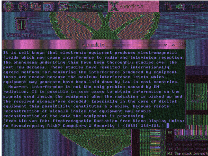
HSV demodulated frame at 12 m, f_c = 350 MHz, B = 40 MHz bandwidth, f_r = 64 MHz, f_s = 3 \times f_p \approx 75.6 MHz resampled rate, 30 frames averaged (coherently)
