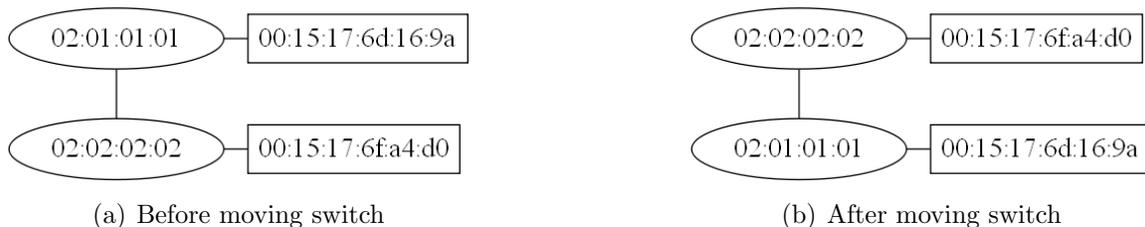
Figure 4.12: Topology of network before (left) and after (right) switch 02:01:01:01 was moved
