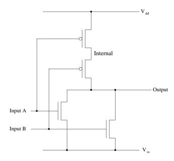
Figure 1: CMOS NOR gate
