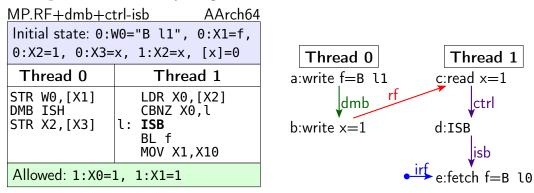
This test includes sufficient synchronisation on each thread to enforce thread-local ordering of data accesses: the DMB in Thread 0 ensures the writes a and b propagate to memory in program order, and the control-dependency into an ISB on Thread 1 ensures the read c and the fetch e happen in program order. However, as we saw in §2, this is not enough to synchronise concurrent modification and execution of code in ARMv8-A. Thread 0 needs the entire
