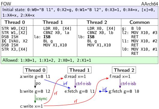
This is not clear in the existing architecture text. It is a case where the architecture design is not very constrained. On the one hand, it has not been observed, and it is thought unlikely that hardware will ever exhibit this behaviour: it would require keeping multiple writes in the coherent part of the data caches, rather than a single dirty line, which would require more complex cache coherence protocols. On the other hand, there does not seem to
