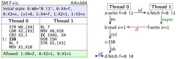
f, Thread 1 fetches the new value and performs just an IC and DSB, before signalling Thread 0 which also fetches f. That IC is not strong enough to ensure that the write is pulled into the instruction cache of Thread 0.
