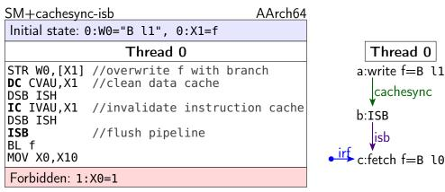
Now the outcome is forbidden. The cache synchronisation sequence DC CVAU; DSB ISH; IC IVAU; DSB ISH (which we abbreviate to a single cachesync edge) ensures that by the time the ISB executes, the instruction and data memory have been made coherent with each other for f. The ISB then ensures the final fetch of f is ordered after this sequence. The microarchitectural intuition for this was in §2; our §4 operational model will describe the semantics of each instruction.
