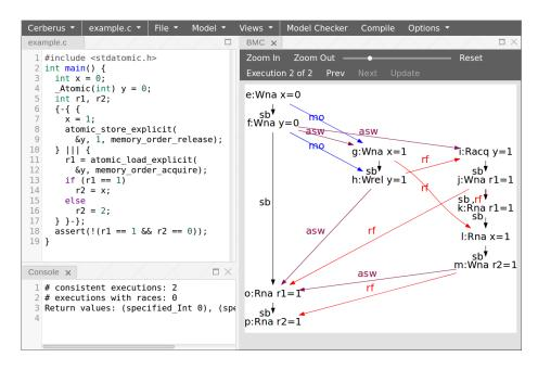
Fig. 1. Cerberus-BMC Screenshot: C11 Release/Acquire Message Passing. If the read of y is 1, then the last thread has to see the write of 1 to x.
