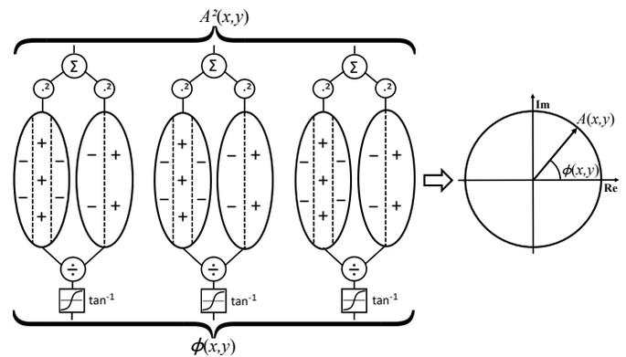
Fig. 2. Demodulation-based encoding of image structure by even- and odd-symmetric phasor modules, resolving both local amplitude  $A(x, y)$  and phase  $\phi(x, y)$  descriptions. From Fig. 14, Daugman and Downing (1995) [18].
