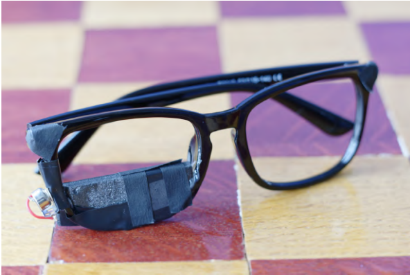
Figure 4.6: Frames of the glasses with an IR LED. The participants were asked to wear these frames to track their head position.
