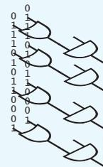
In Serpent's bitslice operation, the bits in the block are "stacked vertically" to a height equal to the width of the ALU. And the move to 64 bit processors will gain us another factor of 2.
