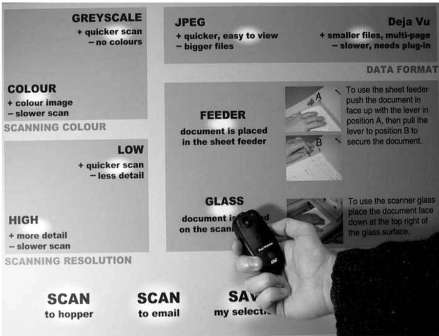
**Figure 2.13.** A smart poster acting as the computerless user interface for a public document scanner nearby. The user is about to scan the document currently on the glass (courtesy of AT&T Laboratories Cambridge).
