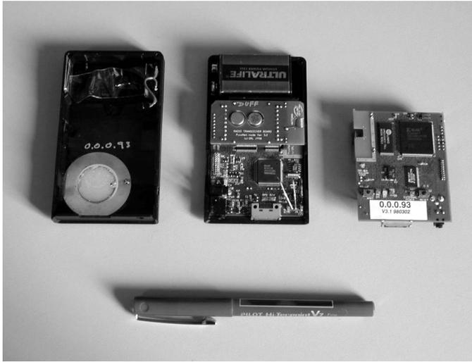
**Figure 2.16.** A PEN node, revealing its insides, and a lowercase pen for size comparison (courtesy of AT&T Laboratories Cambridge).
