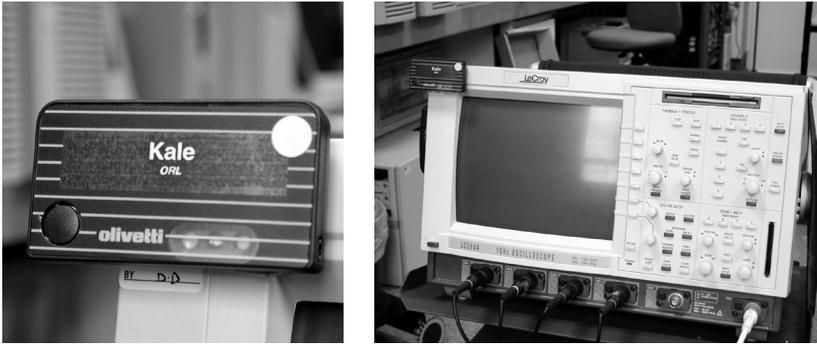
**Figure 2.10.** A tob (“transmit-only badge”) is used to track the location of this trolley-mounted oscilloscope (courtesy of AT&T Laboratories Cambridge).
