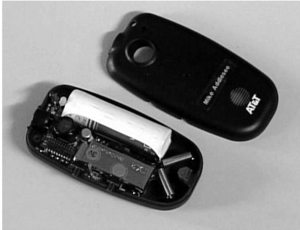
**Figure 2.12.** The Active Bat (courtesy of AT&T Laboratories Cambridge).
