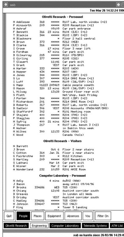
Figure 2.8. The xab application, displaying badge sightings on an X Windows workstation (courtesy of AT&T Laboratories Cambridge).
