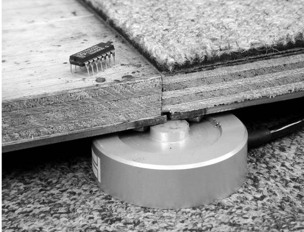
**Figure 2.11.** A detail of the construction of the Active Floor, showing a bare tile, a carpeted tile and a load cell (courtesy of AT&T Laboratories Cambridge).
