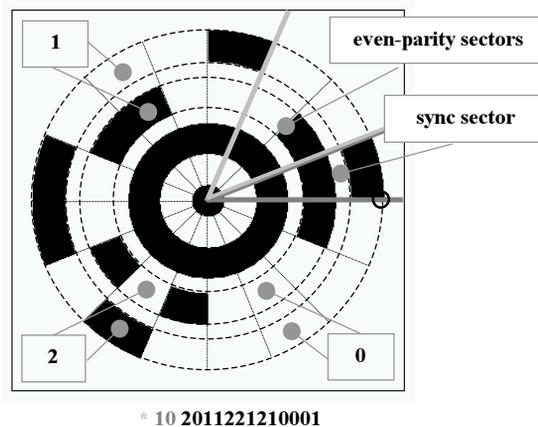
**Figure 2.14.** A TRIP target, showing (anticlockwise from East) the sync sector, the two redundancy sectors and the remaining 13 data sectors, for a total of  $3^{13}$  valid codes (courtesy of AT&T Laboratories Cambridge and Diego López de Ipiña).
