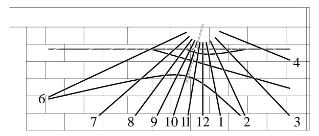
All the markings on the dial are formed by deep V-cuts. Those for the hour-lines are 32mm wide. When the sun shines, the shadow of one edge of a V-cut falls into the depth of the cut and this shadow contrasts starkly with the bright limestone wall. In this way the sun brings the whole dial to life.
