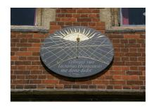
The time indicated by the white hour-lines is the number of hours since sunset. These are called Italian hours. The average of these two times is the time indicated on a normal sundial with a polar-oriented gnomon.
