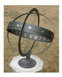
In the Downing armillary sphere, this problem is reduced by making the higher side of equatorial ring thinner than the lower side. It is the lower side which has the hour numbers. In some designs, the higher side of the ring is cut out altogether.
