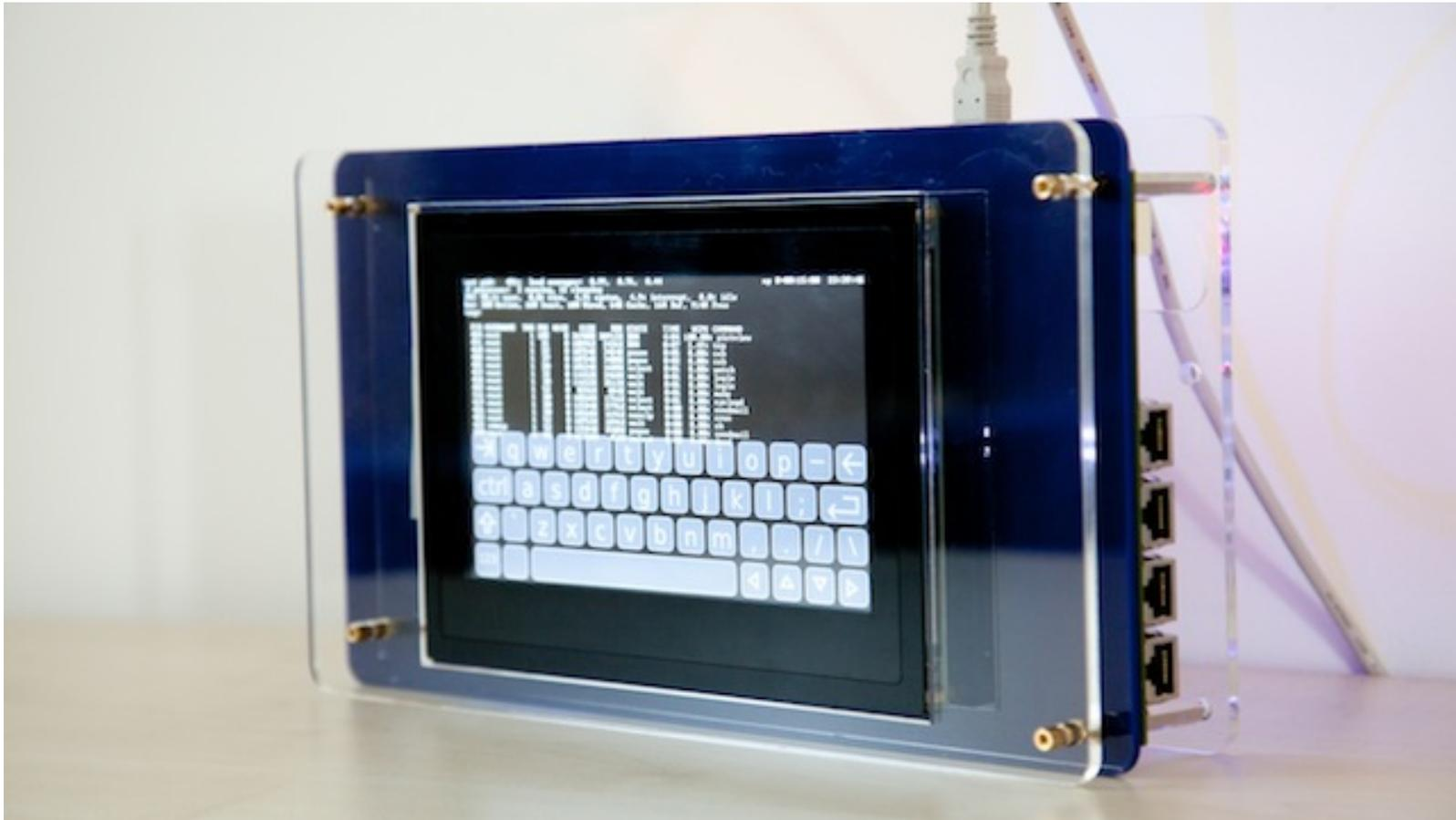
Terasic DE-4 tablet hosting 100MHz CHERI processor, CheriBSD OS
