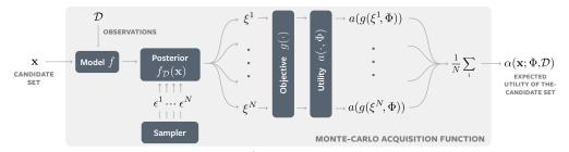
Figure 1: MC acquisition functions. Samples  $\xi_{\mathcal{D}}^i$  from the posterior  $f_{\mathcal{D}}(\mathbf{x})$  provided by the model f at  $\mathbf{x}$  are evaluated in parallel and averaged as in (2). All operations are fully differentiable.
