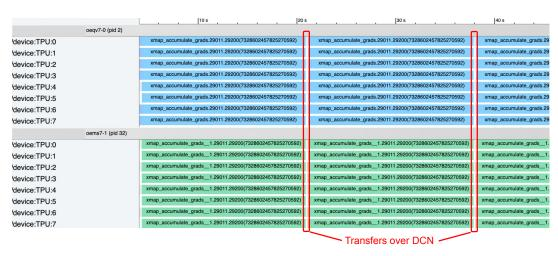
Figure 12. 64B Transformer model training data parallel over two islands of 512 TPUs each. The trace highlights the relatively small overhead of cross-island transfer using DCN.
