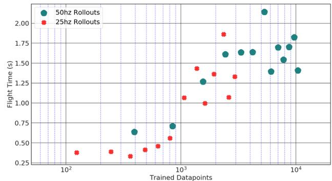
Fig. 12: Mean flight time of each rollout plotted versus the logarithm of the number of available points at train time for each model. The higher control frequency allows the controller to learn faster on wall time, but the plot indicates that there is not a notable difference between control ability when the number of trained points are equal. There is a continuing upward trend of flight time versus training points, but it is difficult to obtain more data in experiment.
