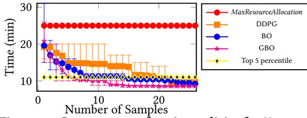
**Figure 16: Convergence of tuning policies for K-means. Each tuner is run 5 times; the mean, min, and max values for the lowest runtime observed so far are plotted.**
