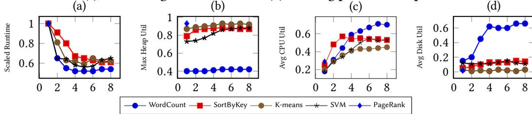
Figure 5: Impact of Task Concurrency on runtime (a), maximum heap utilization (b), average CPU utilization (c), and average disk utilization (d). PageRank runs out of memory for Task Concurrency  $\geq 2$ .
