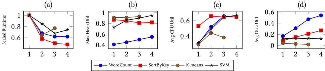
Figure 4: Impact of increasing number of containers per node on runtime (a), maximum heap utilization (b), average CPU utilization (c), and average disk utilization (d). Missing points correspond to instances of failures.
