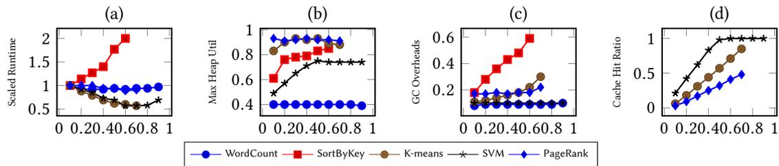
**Figure 6: Impact of Cache Capacity and Shuffle Capacity on runtime (a), maximum heap utilization (b), and average per task GC Overheads (c). X-axis represents Shuffle Capacity as a fraction of Heap for WordCount and SortByKey. On other applications, it represents Cache Capacity. The cache hit ratio is displayed in plot (d).**
