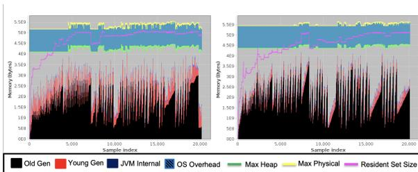
**Figure 9: Comparing memory usage timeline for a container having NewRatio=2 (left) with a container having NewRatio=5. The left side configuration is more prone to failures due to physical memory usage exceeding limit set by resource manager.**
