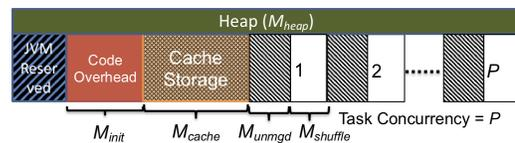
**Figure 3: Heap managed by application framework**
