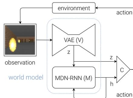
Figure 8. Flow diagram of our Agent model. The raw observation is first processed by V at each time step  $t$  to produce  $z_t$ . The input into C is this latent vector  $z_t$  concatenated with M’s hidden state  $h_t$  at each time step. C will then output an action vector  $a_t$  for motor control, and will affect the environment. M will then take the current  $z_t$  and action  $a_t$  as an input to update its own hidden state to produce  $h_{t+1}$  to be used at time  $t + 1$ .
