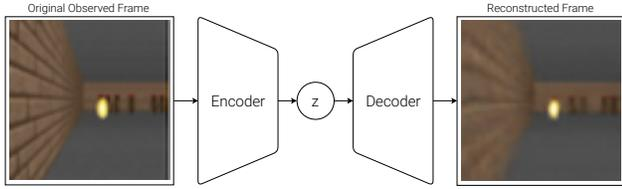
Figure 5. Flow diagram of a Variational Autoencoder (VAE).
