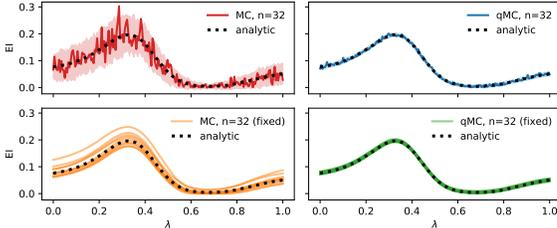
Figure 2: MC and QMC acquisition functions, with and without (“fixed”) re-drawing base samples between evaluations. The model is a GP fit on 15 points randomly sampled from  $\mathbb{X} = [0, 1]^6$  and evaluated on the Hartmann6 function. Evaluation is along the slice  $x(\lambda) = \lambda \mathbf{1}$ .
