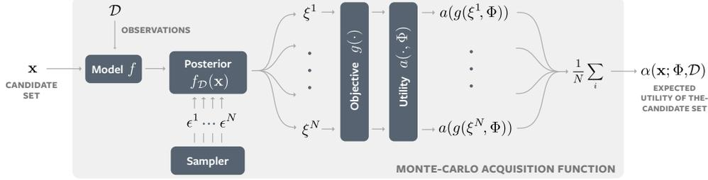
Figure 1: MC acquisition functions. Samples  $\xi_D^i$  from the posterior  $f_D(\mathbf{x})$  provided by the model  $f$  at  $\mathbf{x}$  are evaluated in parallel and averaged as in (2). All operations are fully differentiable.
