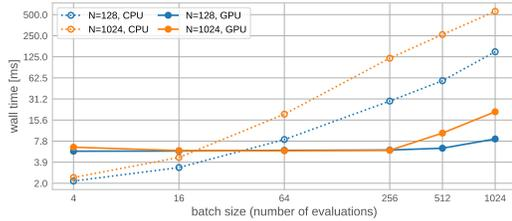
Figure 6: Wall times for batched evaluation of qEI
