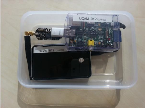
Figure 3: Raspberry Pi OpenBeacon Reader
