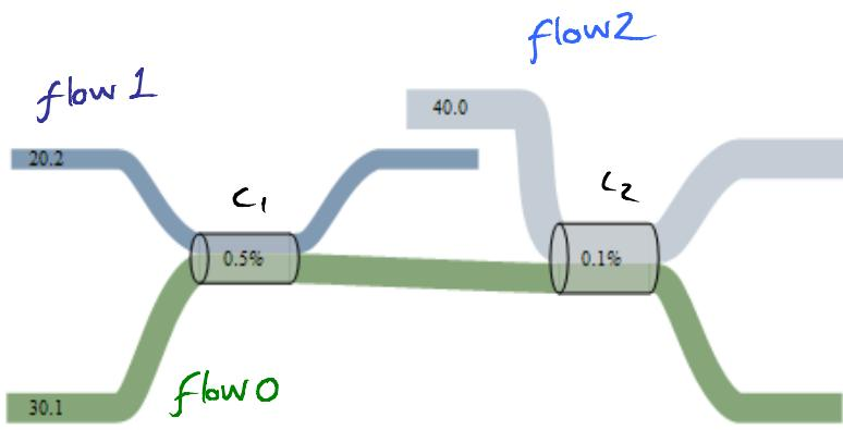
Example: maximize  $\frac{-2}{RTT_0^2 y_0} - \frac{2}{RTT_1^2 y_1} - \frac{2}{RTT_2^2 y_2}$
