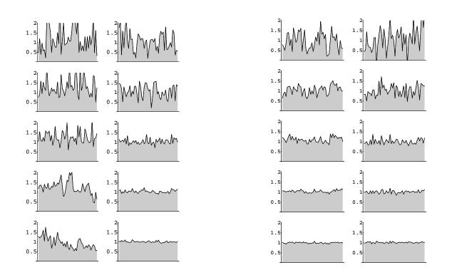
**Left.** Internet traffic (left) is bursty at all timescales, while a traditional Gaussian traffic model (right), matched to have the same mean and variance, is not. The top plots have the finest time-scale; each subsequent plot shows a four-fold longer time-scale.
