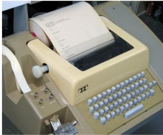
Figure 1.13: Teletype/teleprinter: These devices were almost entirely mechanical with the electric circuit being little more than one switch activated by cams for transmit and one solenoid for receive.
