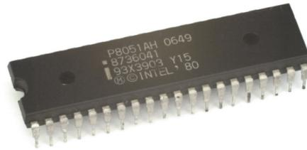
Figure 1.5: Intel 80C51 Microcontroller Chip from 1980.
