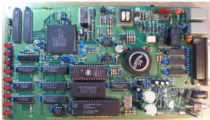
Figure 2.34: PCB of a similar modem - but offchip RAM and ROM for the 80C31 microcontroller.
