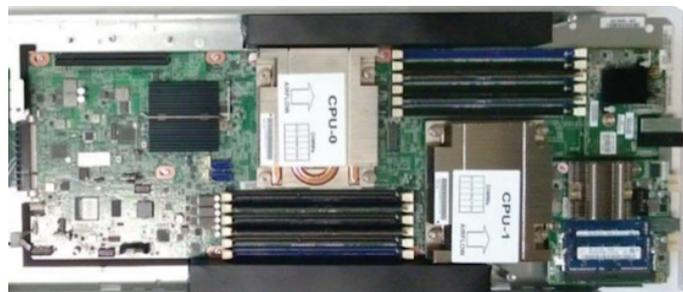
Figure 10.5: Catapult Blade - FPGA is at the lower right, its heatsink visible above its blue DRAM DIMMs.
