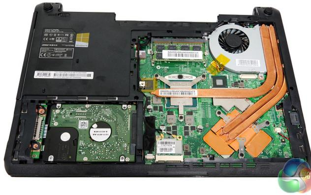
Figure 2.23: Thermal management heat pipes in a modern laptop.
