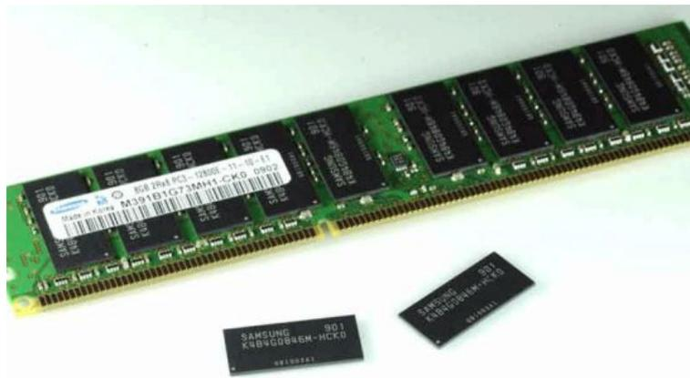
Figure 2.9: DRAM single-in-line memory module (SIMM).
