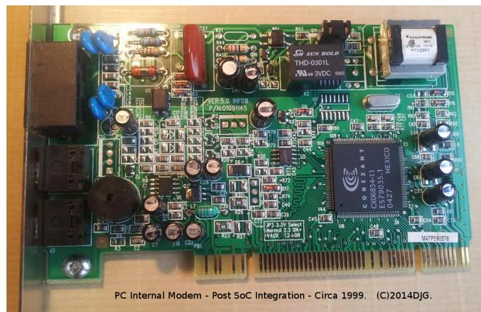
Figure 2.37: PCB of a similar modem - Post SoC technology.
