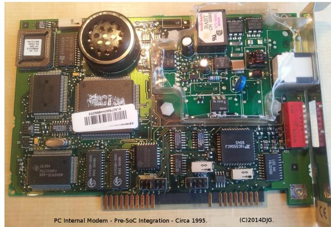
Figure 2.36: Modem NIC (network interface card) Pre-SoC integration.
