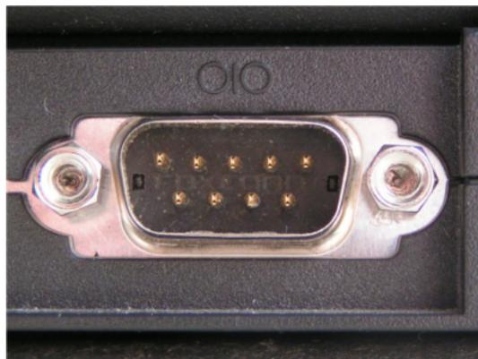
Figure 1.12: Serial Port Connector (9 pin instead of original 25 pin).
