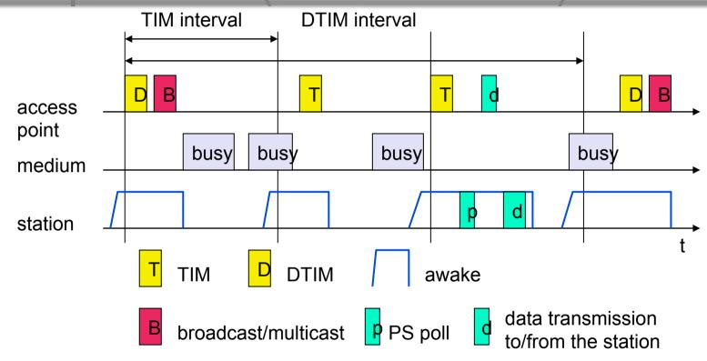
TIM: list of stations for which there will be data in the slot DTIM Interval indicates the delivery traffic indication map: for broadcast and multicast frames. It's a multiple of TIM
