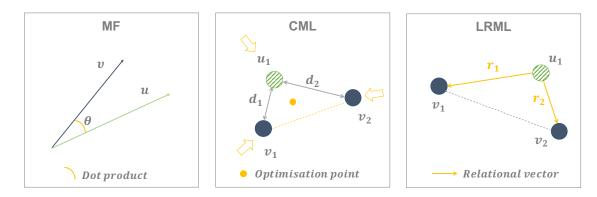
Fig. 2.2 Geometric comparisons of MF, CML, and LRML recommendation algorithms. MF-based methods calculate the dot product of user and item vectors; CML minimises the Euclidean distance between positive user-item pair, and; LRML learns a relational vector for each user-item pair.
