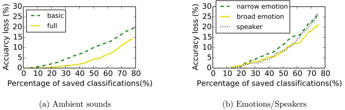
Figure 3.4.4: The percentage of misclassified sounds/ emotions/ speakers as a function of the proportion of saved GMM classifications due to engaging the similarity detectors. The similarity between subsequent sounds is computed based on two cases for the ambient sounds: the basic (without MFCC) and full set of features (with MFCC).
