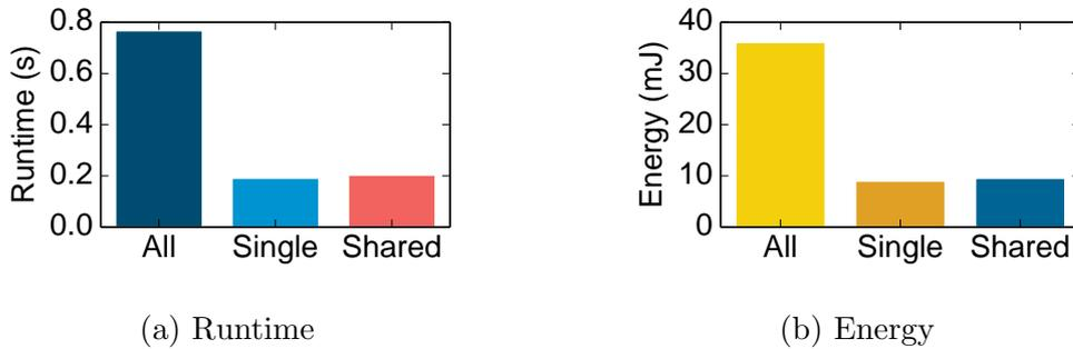
Figure 4.5.3: Runtime and energy for performing DNN classification on the low-power Hexagon DSP when all single models (All), a single model (Single), or the DNN with shared hidden layers (Shared) are run. Single models are run sequentially where each model does each task separately, and the shared one leverages the multi-task design to output all inferences.
