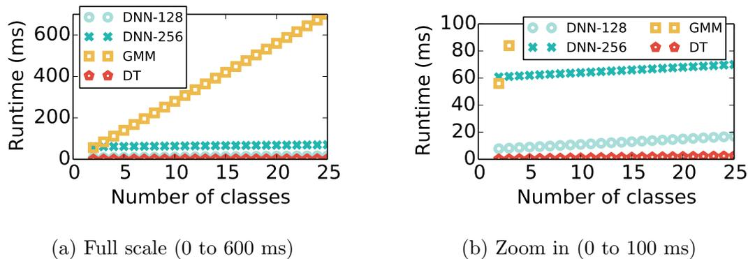
Figure 4.4.3: DSP runtime of the inference stage of the various classifiers as a function of the number of classes. The results suggest that DNNs scale extremely well with the increase in the number of classes, in a manner similar to a DT, while often providing superior accuracy.
