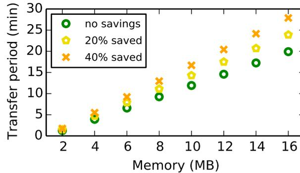
Figure 3.4.5: Time in minutes before the CPU is woken up by the DSP as a function of the runtime memory constraint on the co-processor. The additional gain in time is also given when the similarity detectors eliminate a percentage of the classifications by propagating class labels, discarding features and thus freeing space.
