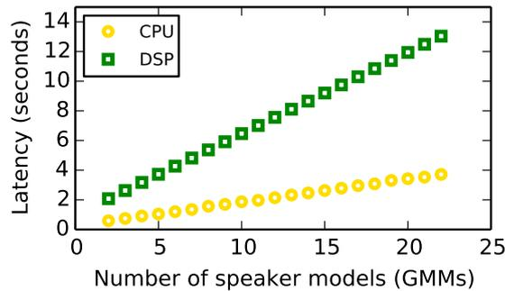
Figure 3.4.3: Runtime of the emotion and speaker recognition use cases as a function of the number of GMMs.
