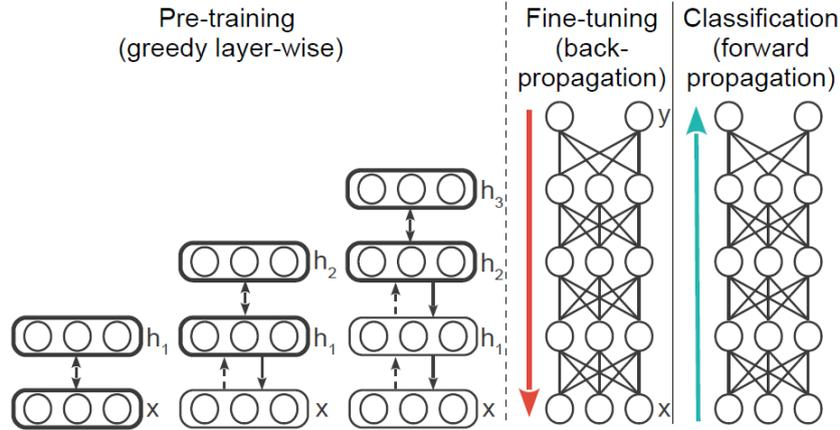
Figure 2.2.2: Example phases of building a Deep Neural Network with 3 hidden layers ( $h_1$ ,  $h_2$ , and  $h_3$ ), input layer  $x$  and output layer  $y$ . Shown are the pre-training, fine-tuning and classification phases of a DNN variant called a Deep Belief Network.
