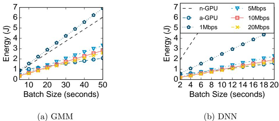
Figure 5.6.3: End-to-end energy as a function of the batch computation size for running the audio pipelines on the GPU vs cloud offloading. Legend is shared.
