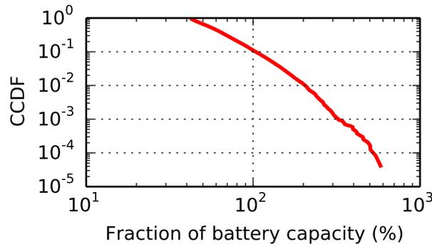
Figure 3.4.8: Complementary cumulative distribution function (CCDF) of the percentage of battery capacity drained in 24 hours of smartphone usage. It shows the proportion of time users will exhaust battery at least the percentage shown on the x axis during the day. Percentages greater than 100% mean that the mobile user needs to recharge the battery at least once during the day.
