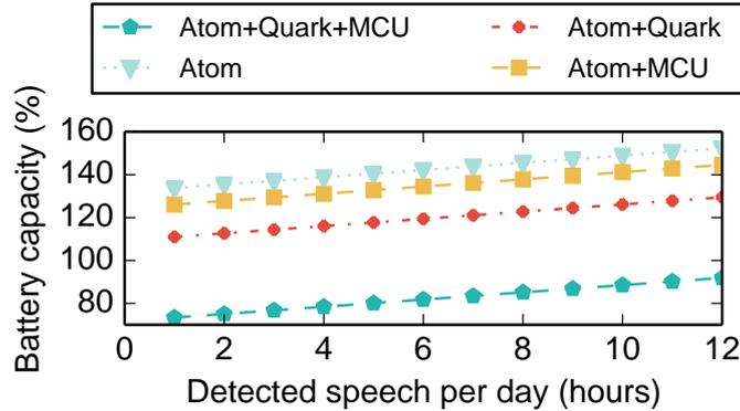
Figure 3.5.1: Percentage of the battery needed to handle the sensor processing of a daily workload (8h of silence, 1h to 12h of speech, 20 questions per day). Values higher than 100% indicate the battery needs to be recharged at least one more time during the day to sustain the workload.
