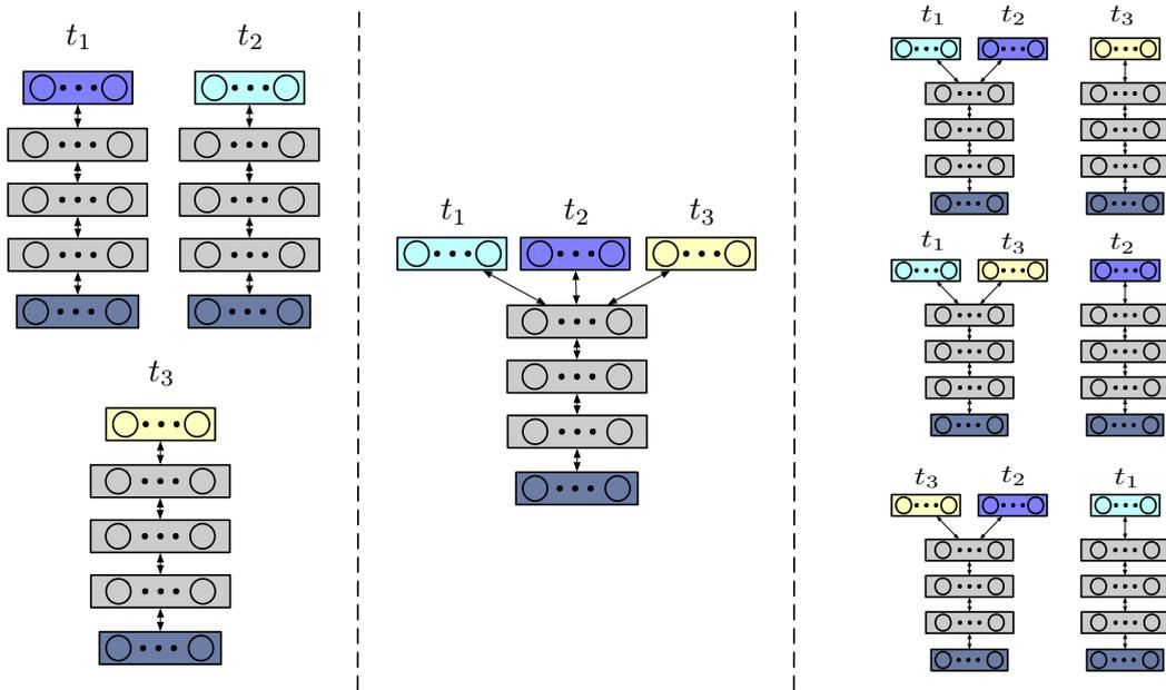
Figure 4.5.2: Different deployment configurations for 3 audio analysis tasks ( $t_1$ ,  $t_2$ , and  $t_3$ ). We can have independent models for each task (left), all tasks can share the layers of the DNN (middle), or we can deploy a pair of tasks with a shared representation and a task with an independent model (right).
