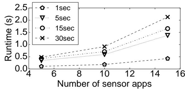
Figure 6.5.1: Runtime of the scheduling algorithm as a function of the number of apps and the length of the rescheduling interval.
