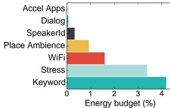
Figure 3.5.2: Breakdown of the energy consumed by the various system component computations for the workload scenario of 4.5h of speech, 11.5h of ambient context, 15min WiFi duty cycle and 20 dialogue commands per day. The reported energy budget reflects the additional energy of the raw processing on top of what the Atom CPU consumes in an active state.
