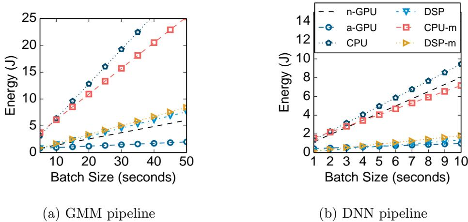
Figure 5.6.1: Energy (J) as a function of the audio processing batch size in seconds. Legend is shared, axis scales are different.
