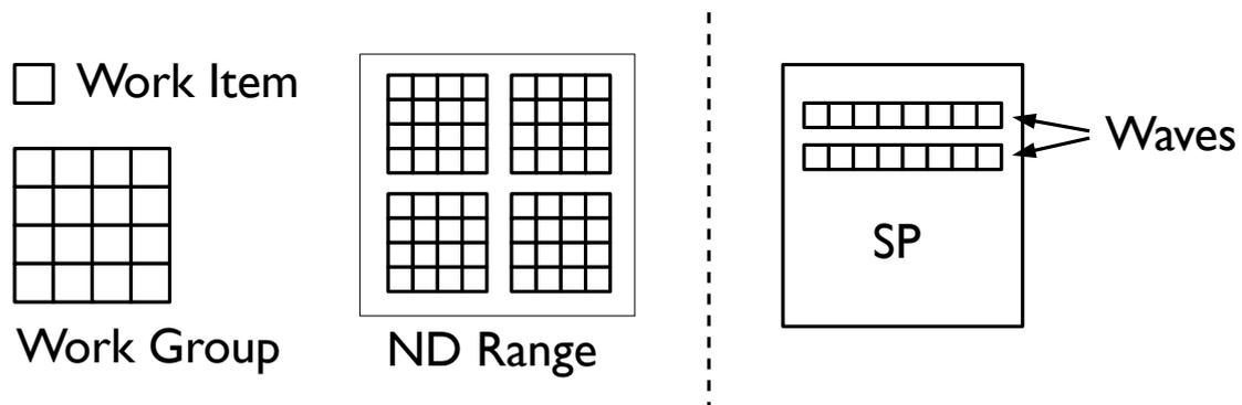
Figure 5.2.1: OpenCL thread model and a GPU Shader Processor. The SP features 2 waves of 8 work items each, it can run 16 threads in total simultaneously. The work items of one work group are executed on a single SP.
