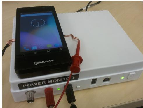
Figure 3.3.1: Snapdragon 800 Mobile Development Platform (MDP) [46] used for the system development.
