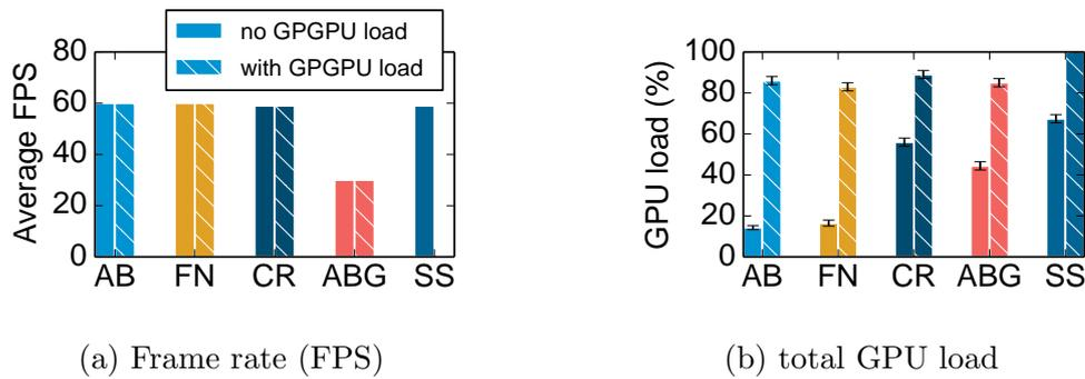
Figure 5.6.5: Average frame rate and GPU load when the games run without and with additional GPGPU load. Games in the experiment are Angry Birds (AB), Fruit Ninja (FN), Crossy Road (CR), Angry Birds GO (ABG), and Subway Surfers (SS). Legend is shared.
