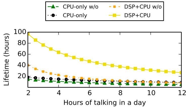
Figure 3.4.6: Lifetime in hours of the system running on the CPU only or the DSP+CPU as a function of the proportion of detected speech during a 24-hour day. Two versions of the system are provided: without (w/o) and with optimisations.
