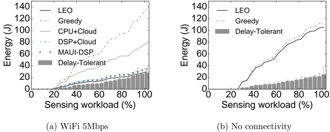
Figure 6.5.3: Energy consumption of the offloading strategies compared against the delay-tolerant LEO as a function of the sensing workload saturation for the medium load scenario (M).
