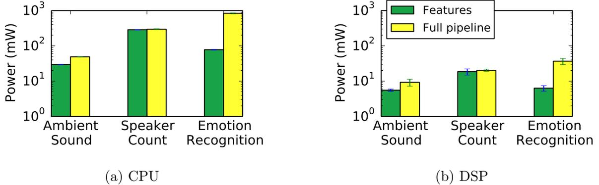
Figure 3.4.2: Average power consumed by the various apps when running on (a) the CPU and (b) the co-processor. Values on the Y axis are in a logarithmic scale.
