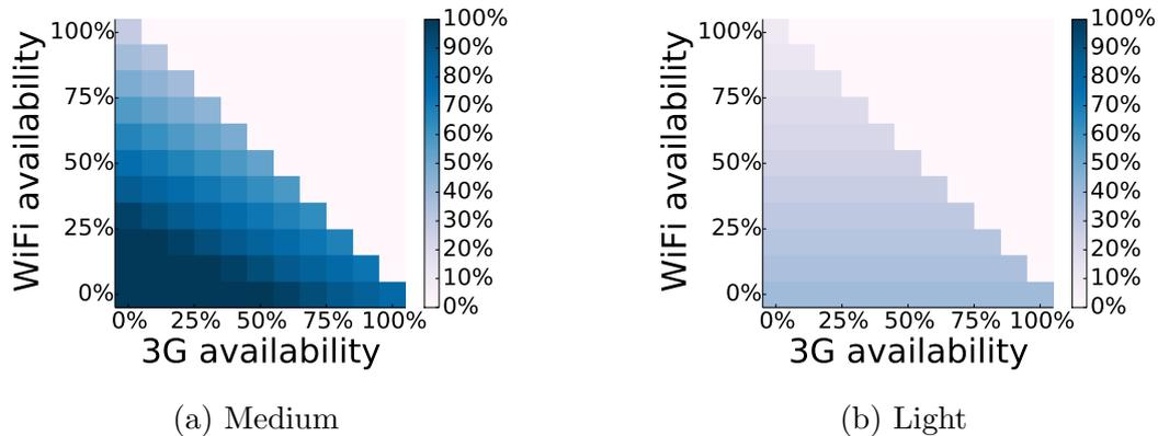
Figure 6.5.4: Percentage of the battery capacity needed for processing 4.5 hours of sensing context under varying network availability.
