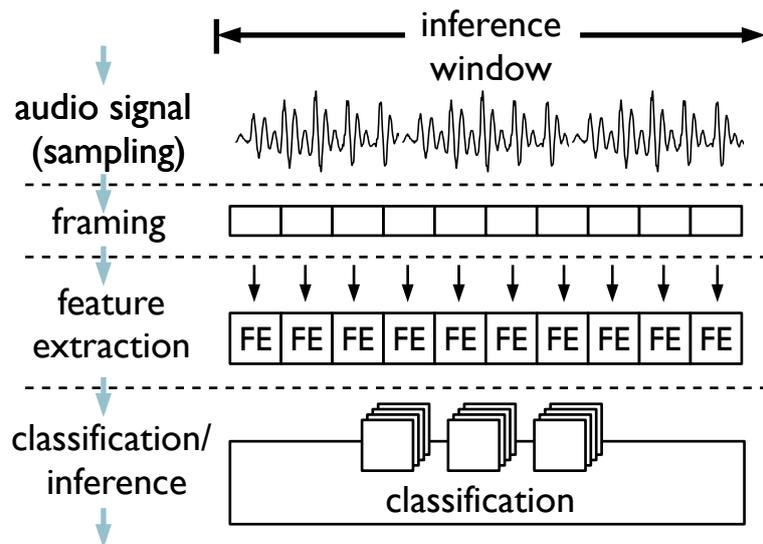
Figure 2.2.1: Audio pipeline structure.
