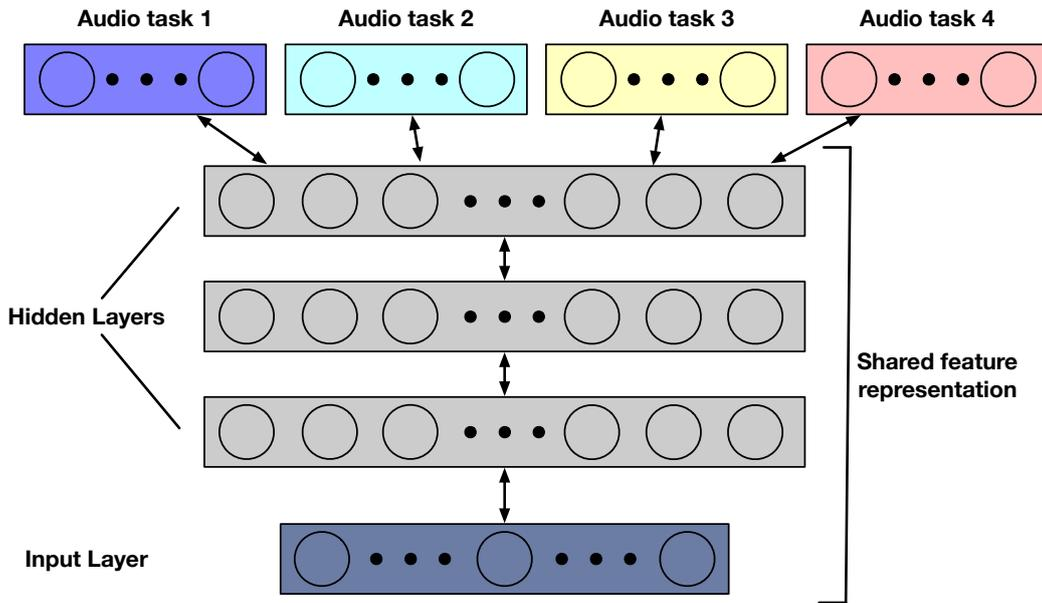
Figure 4.5.1: Architecture of the multi-task DNN.
