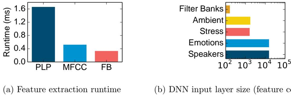
Figure 4.4.1: (a) Runtime needed to compute features from one 30ms frame. (b) Size of the DNN input layer (number of features per audio processing window) across the various audio sensing tasks compared against the use of window-agnostic summary filter banks (FB).
