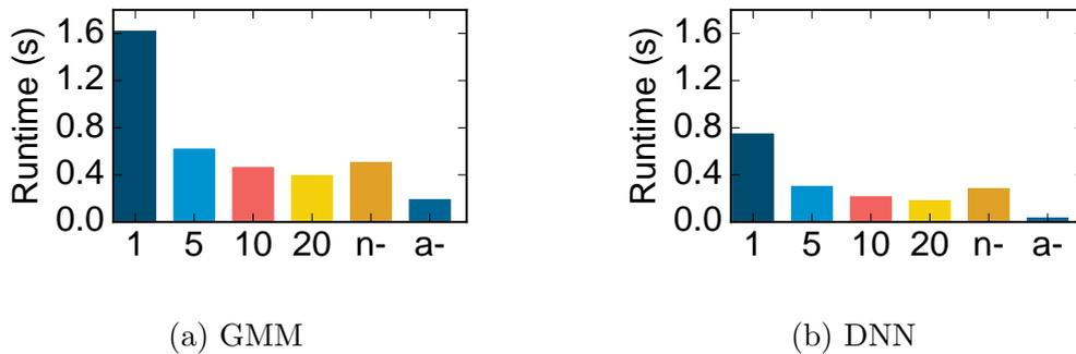
Figure 5.6.2: End-to-end latency for computing the audio pipelines on the GPU vs cloud. Numbers on the x axis show throughput in Mbps, and n- and a- refer to n-GPU and a-GPU.
