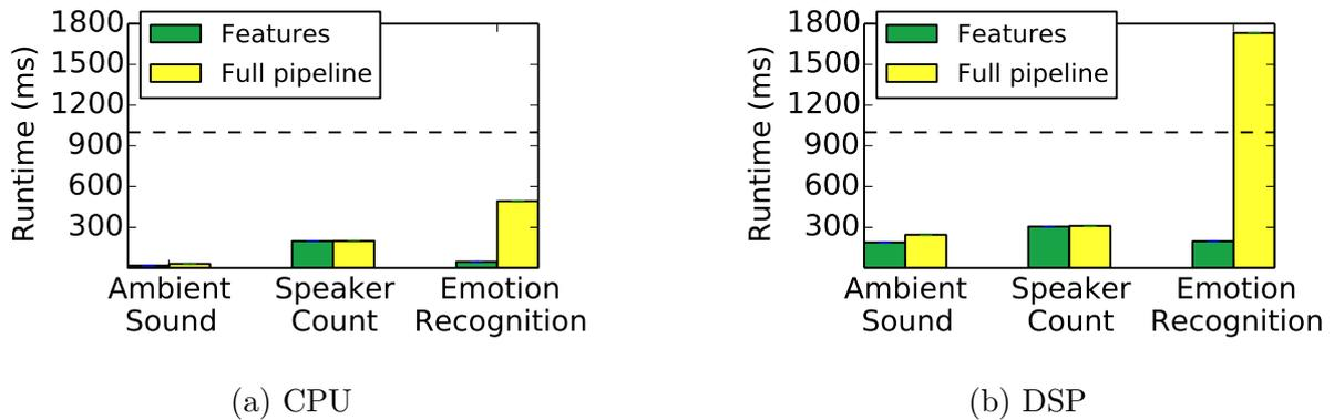
Figure 3.4.1: Normalised runtimes per one second of audio sensing for the various apps when execution happens on (a) the CPU and (b) the co-processor. Note that the Speaker Identification pipeline (not shown) shares the same algorithmic components as Emotion Recognition, the results are qualitatively the same modulo the total number of GMMs used.
