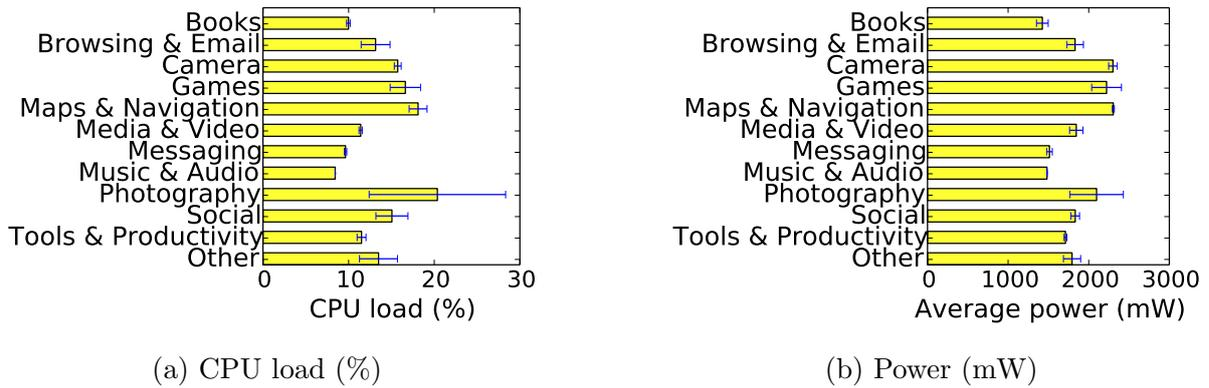
Figure 3.4.7: The average (a) CPU load and (b) power of interactively (screen on) running apps from the given categories.
