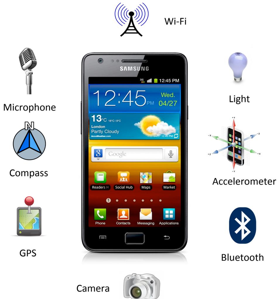
Figure 2.1: Sensors embedded in the Samsung Galaxy SII mobile phone.
