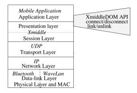
Figure 1. The protocol stack for mobile environments using XMIDDLE.
