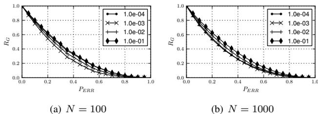
Fig. 4. Temporal robustness  $R_G$  as a function of probability of error  $P_{ERR}$  in the ER random model for different link probability  $p$ . The size of the system has no impact on temporal robustness: furthermore, the system fails smoothly as the probability of error increases.
