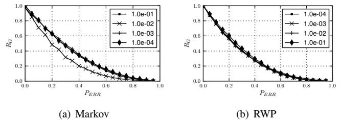
Fig. 5. Temporal robustness  $R_G$  as a function of probability of error  $P_{ERR}$  and for different values of  $P_{ON}$  for the Markov-based and for the RWP random model (RWPG does not deviate from RWP)
