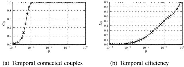
Fig. 1. Fraction of connected couples of nodes  $C_G$  (a) and temporal efficiency  $E_G$  (b) as a function of link probability  $p$  for a temporal ER graph with  $N = 100$  nodes and with  $T = 100$ . Simulation results are averaged over 100 runs.
