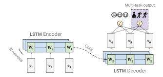
Figure 3: LSTM Encoder-Decoder model. The mood sequence  $(v_1,v_2,v_3)$  passes through an LSTM (states  $W_1$ ), gets transformed to a single vector (dotted) and decoded through another LSTM  $(W_2)$  that predicts future mood sequences  $(v_4,v_5,v_6)$ . Two fully-connected layers are applied to every time-step of the output (yellow circle), one for valence and one for arousal (purple box).
