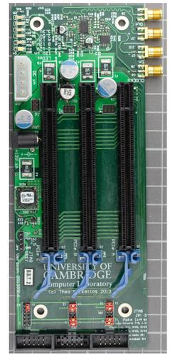
Fig. 8. PCB for BlueLink over PCIe connectors
